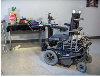
Fig. 1. The Playbot wheelchair which we used in our experiments.
